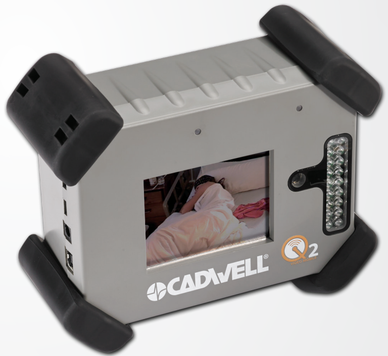
Q-Video Mobile 2 has infrared lights for low-light recording
